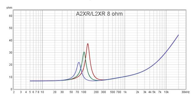
Picture shows impedance with optional 3-way resonance switch
